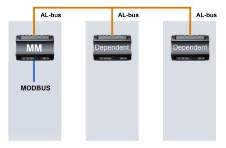
With the cascade manager you have a good control of all boilers. With a Modbus connection to the managing boiler you can access all data from the Managing boiler, and following data from Dependents:
